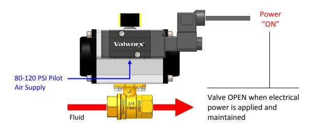
Notes: 1) Spring return on-off control valves can be setup normally open and fail open if required. 2) The manual override can be used to open or close the on-off valve, provided the pilot air supply is maintained.
