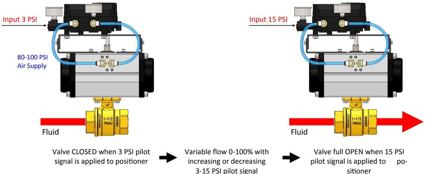
Notes: Double acting actuators will fail closed with loss of control signal, provided air supply pressure is maintained. Double acting actuators will fail in-place (may drift) with loss of air supply pressure. Standard spring return actuators will fail closed with loss of air supply pressure or control signal (failsafe). Spring return valves can also be setup to operate in reverse mode (4mA or 3 PSI = open) and fail open if required.
