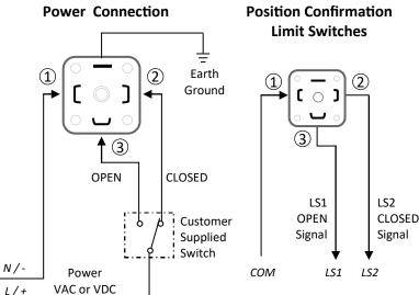
Wiring Main Power Connection: Power is connected to the actuator via the large gray DIN plug connector. Wires are connected to screw terminals located inside the connector. User/installer to supply a three way switch, control relay, PLC or other suitable switching device to control the actuator position.
