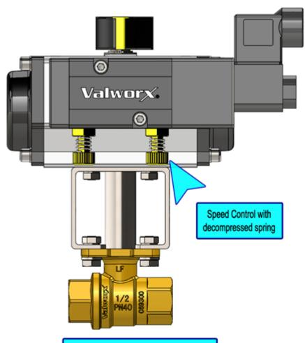
Springs can be tightened by hand to close off and reduce output of air, or loosened to allow nearly full speed flow of exhaust.
