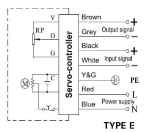
Actuated Valves with EPS Positioner DC Voltages
